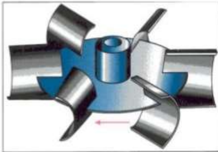
Radial Flow turbine
